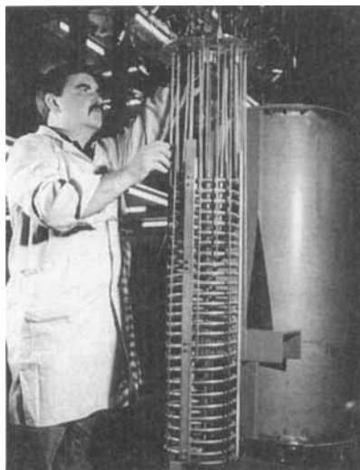
FIGURE 3. Tubular reactor of the 10-kg SCWO facility.
